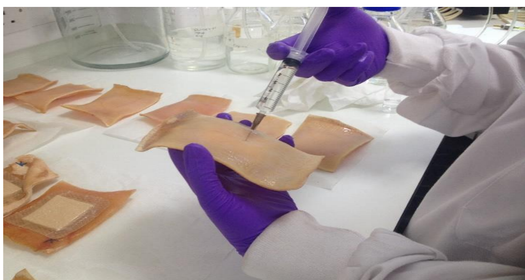
Figure 1. A photograph demonstrating phosphate buffered saline being injected into a porcine skin explant prior to peel force assessment.
